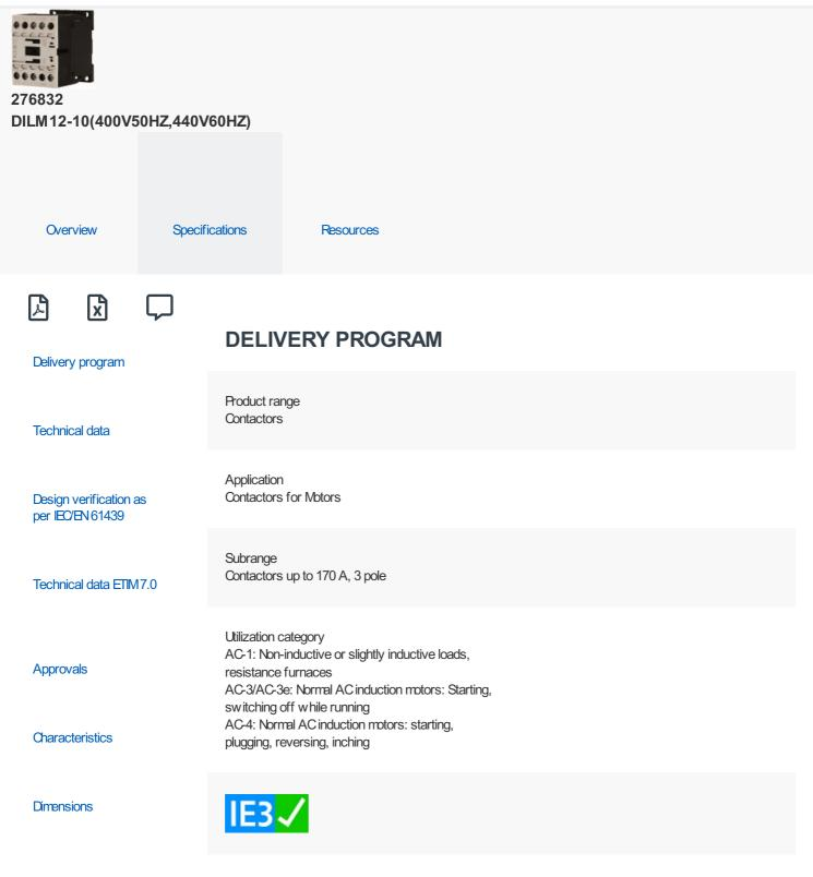
Notes Also suitable for motors with efficiency class IE3. Connection technique Screw terminals
